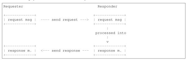
The above shows the four message instances involved in communication between an aiocoap client and server process. Boxes represent instances of Message, and the messages on the same line represent a single CoAP as passed around on the network. Still, they differ in some aspects:
