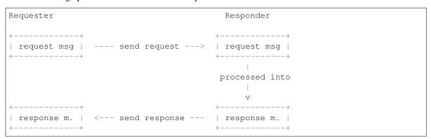
The above shows the four message instances involved in communication between an aiocoap client and server process. Boxes represent instances of Message, and the messages on the same line represent a single CoAP as passed around on the network. Still, they differ in some aspects:
